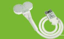
Butterfly Coil 70mm with controls Typical use: Focused cortical stimulation, mainly for rTMS.
